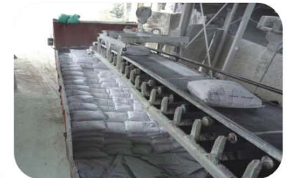
Automatic belt loading
